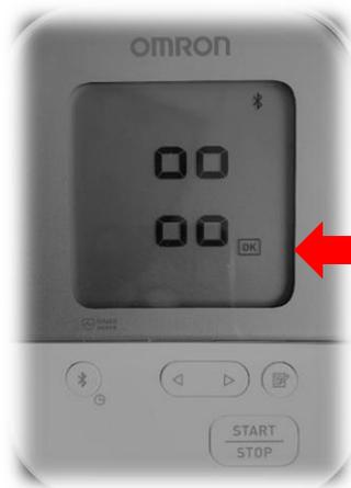
After few seconds, OK displays on screen to confirm it was connected successfully
